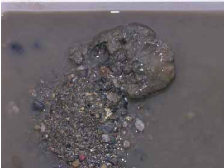
Photograph 48 (left). Straight Creek sediment sample had significantly more sand than very fine sand, silt and clay.
