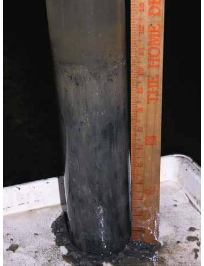
Photographs 46-47. Cove 8. Sample points one and three (left and right) had significantly more of the smallest size grains than gravel.
